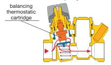
When thermal disinfection is used for legionella growth protection, the function is activated by a second thermostatic by-pass cartridge that opens at 160°F, opening to allow flow for the disinfection process independent of the almost-closed balancing thermostatic cartridge.
