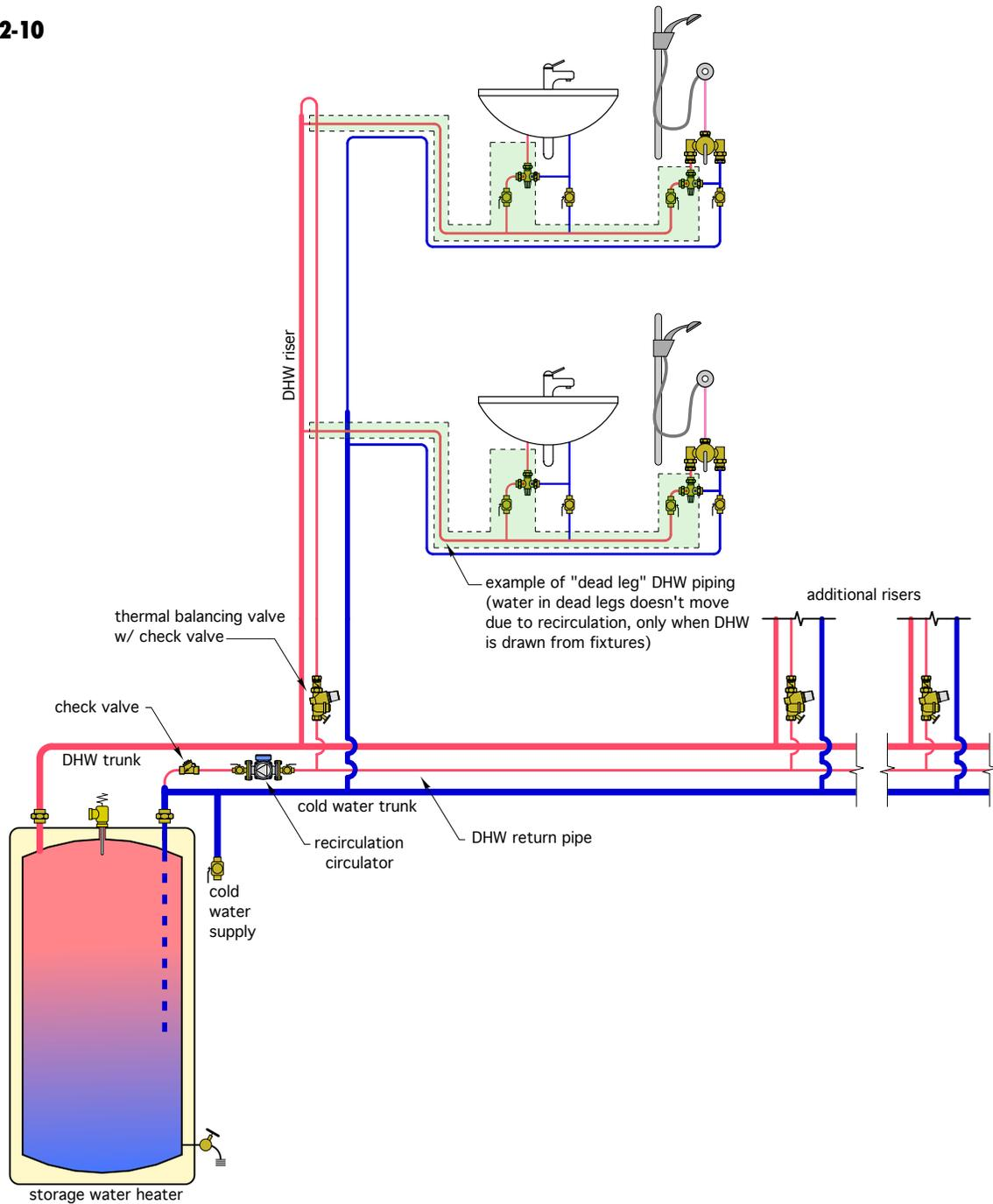
to stagnate in pipes connected between that loop and the fixtures. These pipes are often referred to as “dead legs” in the system. Figure 2-10 shows the concept.
