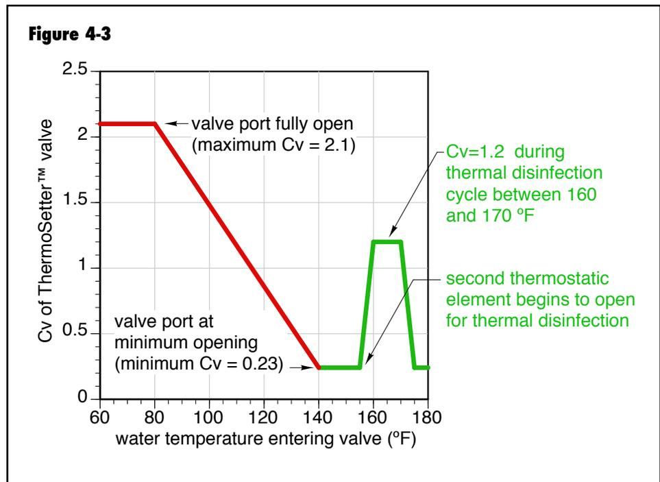
thermal balancing valve with integral check valve within each of the recirculation return piping paths.
