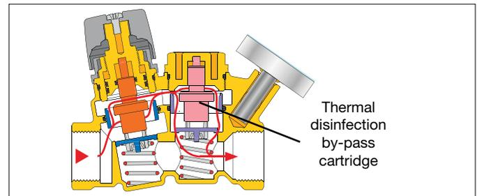
Alternately, the 1163 series models incorporate a by-pass valve for thermal disinfection which is activated by a optional field mounted thermo-electric actuator, code 656 series, controlled by an automation system.
