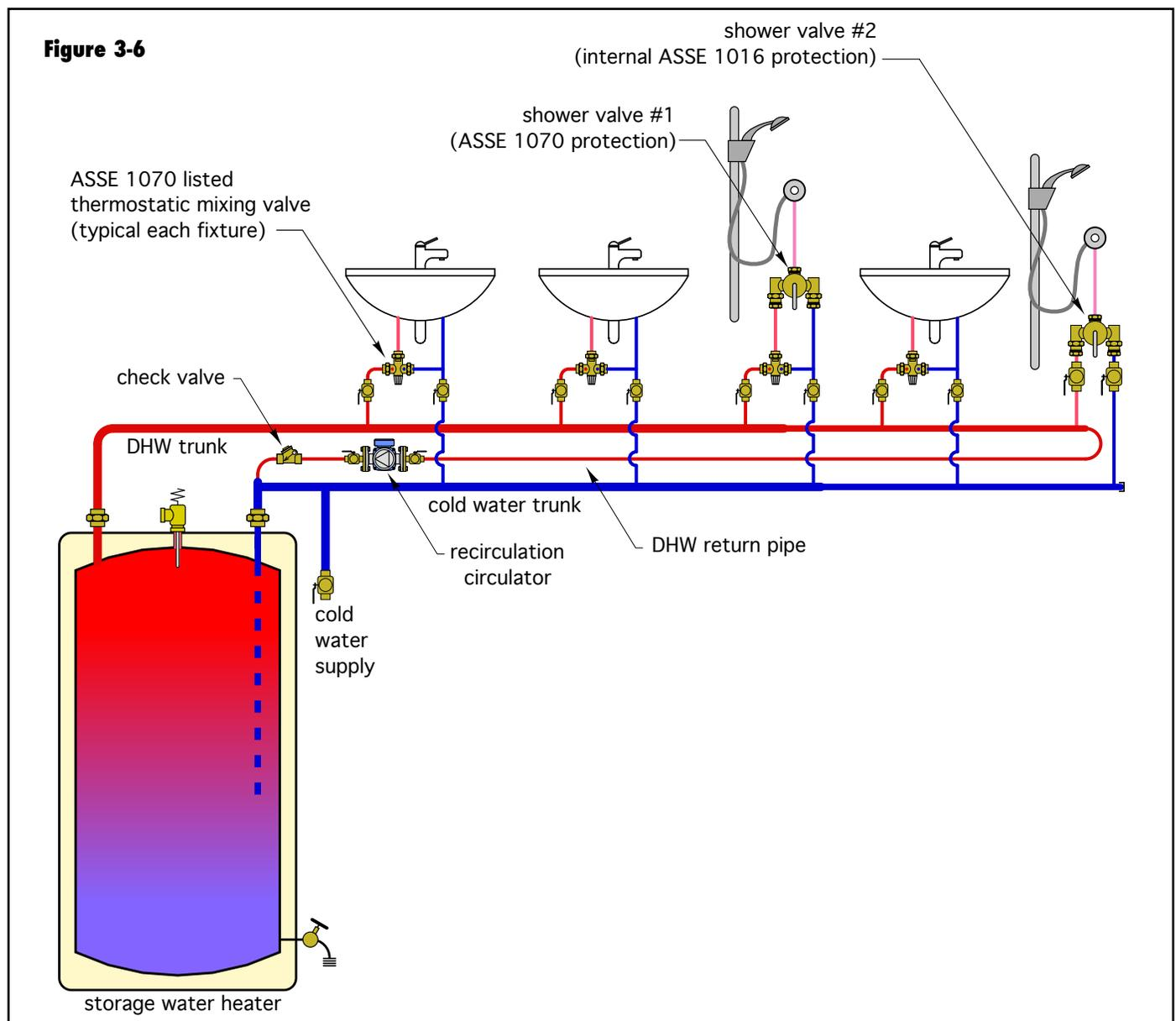
Four of the five fixtures in Figure 3-6 have ASSE 1070 anti-scald mixing valves installed in close proximity to the fixture. The shower valve at the far right of the system has an internal temperature compensating mechanism conforming to ASSE 1016, and as such does not require an ASSE 1070 mixing valve.
