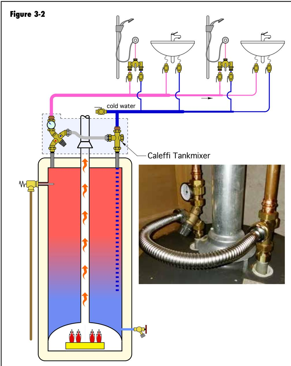
In this system, which does not have downstream devices to further reduce water temperature, the outlet temperature from the thermostatic mixing valve would typically not be set above 120°F. Even lower outlet temperature settings such as 110°F may be required in some circumstances.
