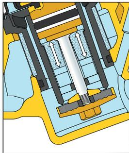
The special cross-section of the flow path between the seat and shuttle seal stabilizes upstream pressure fluctuations and high flow rates, reducing noise levels caused by the flowing water.
