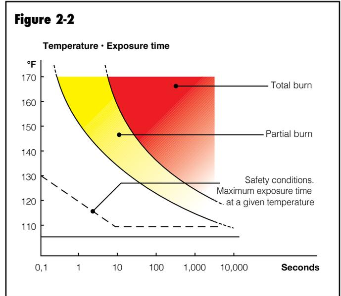
While it may seem intuitive to never set the temperature controls that regulate domestic water heating above a maximum safe temperature, such as 110°F, there are circumstances where this is not possible.
