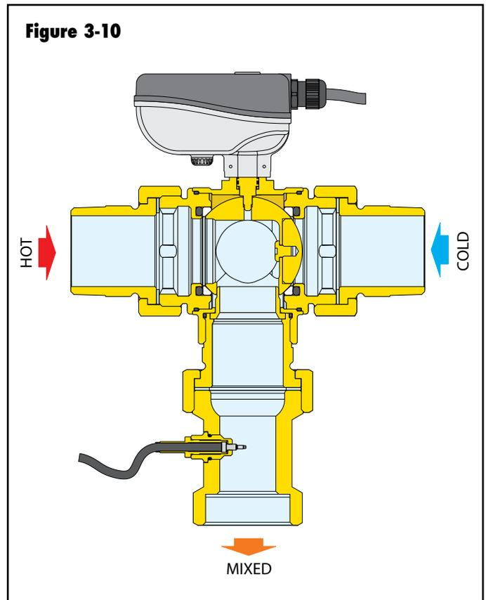
This valve uses a rotating ball to control the proportions of entering hot and cold (or warm) water. The ball is rotated by the motorized actuator at the top of the valve. The mixed flow then passes a temperature sensor, which provides the controller with continuous feedback of leaving water temperature.
