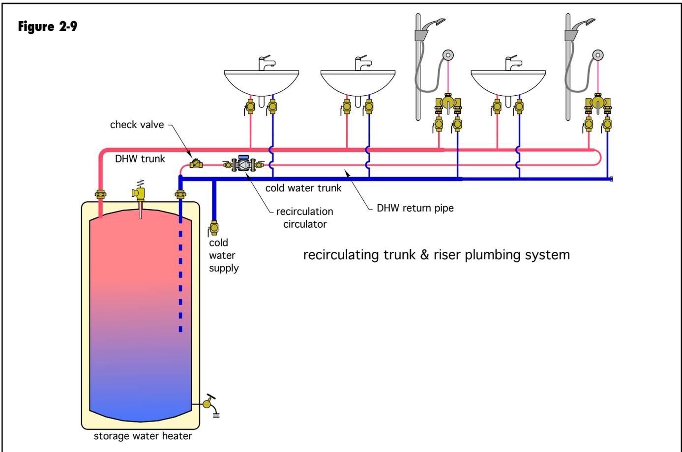
of the system, which, depending on the operating times of the circulator, reduces the potential for stagnant water.
