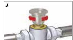
Temperature adjustment cap in place
