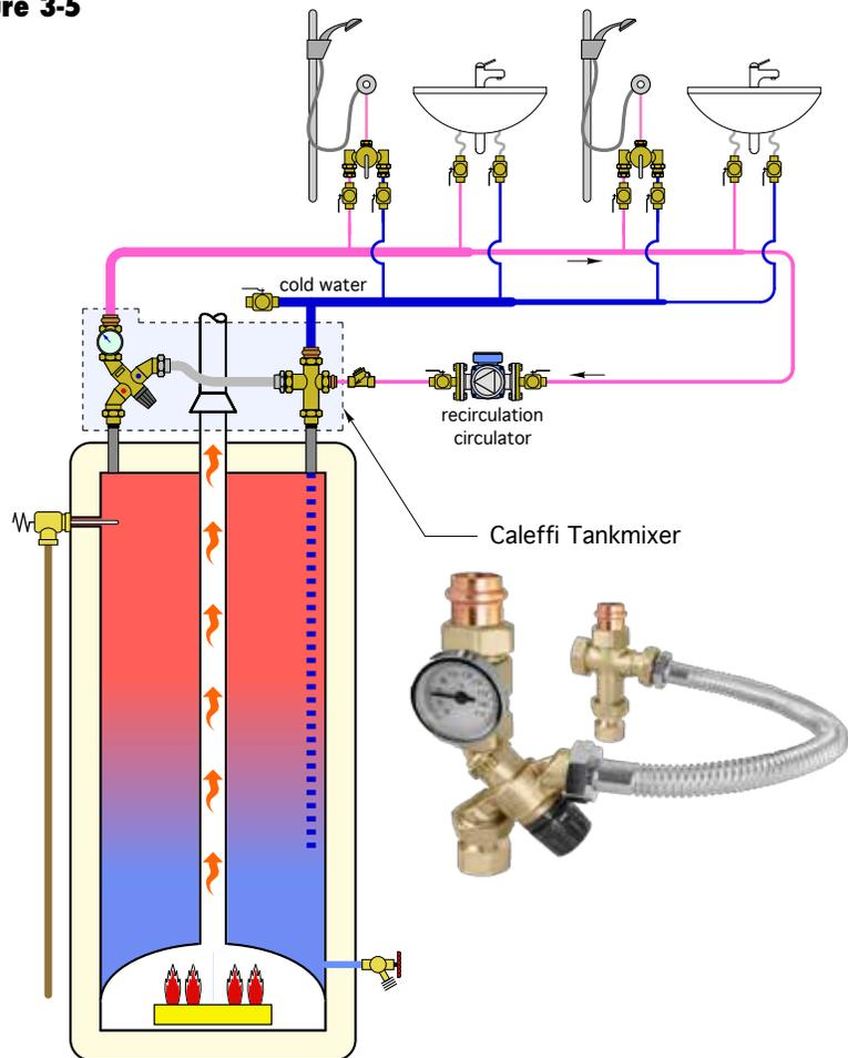
A small stainless steel or bronze circulator has been added to the system, along with piping that carries domestic hot water that has reached the farthest fixture back to the water heater. The same Caleffi TankMixer assembly shown in Figure 3-2 can be used in this application. The cap that covered the side port of the cold water fitting as shown in Figure 3-2 is removed, and the recirculation pipe is connected to this port.
