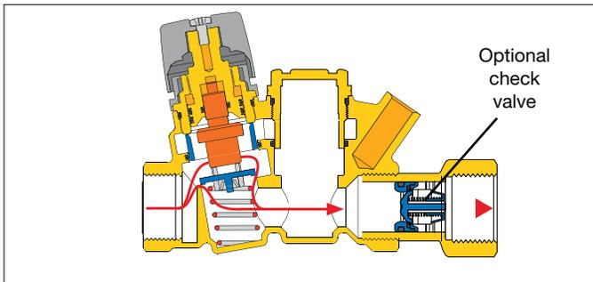
For systems using thermal disinfection for Legionella growth protection, the 1162 series models incorporate a second thermostatic by-pass cartridge that activates at 160°F. A second flow path opens providing flow for the disinfection process which is independent of the primary balancing cartridge.
