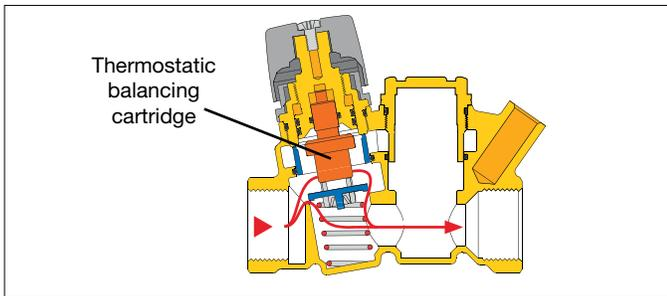
Optional check valve is available for all models, which protect against circuit thermo-syphoning.
