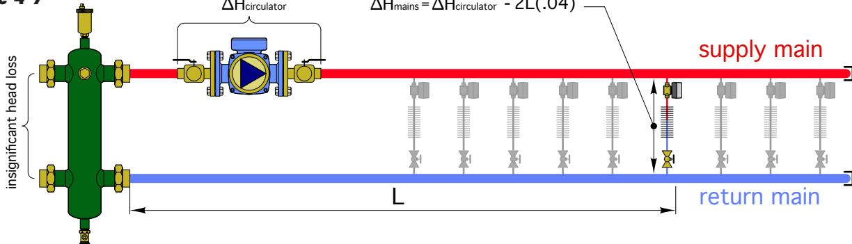
$$\Delta H_{\text{mains}} = \Delta H_{\text{Piping+HE}} + \Delta H_{\text{BV}}$$
