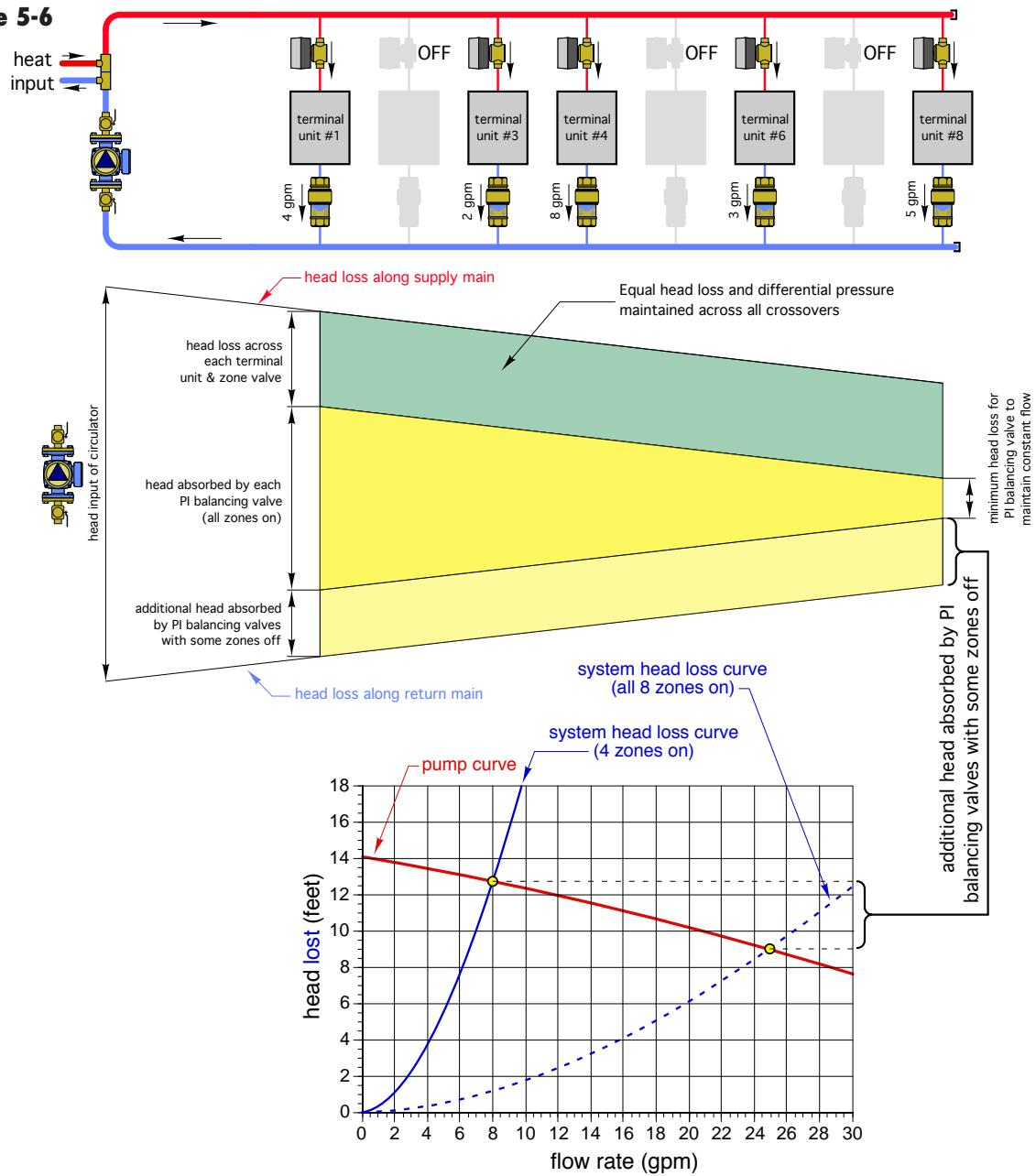
added to the system when a variable-speed pressure-regulated circulator is used.
