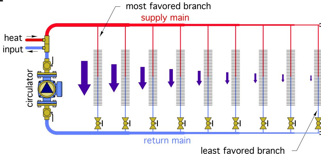
Although balancing to establish a set of predetermined flow rates is not guaranteed to produce perfect comfort in all spaces, it certainly is a means toward that end, and thus an essential part of modern hydronics technology.
