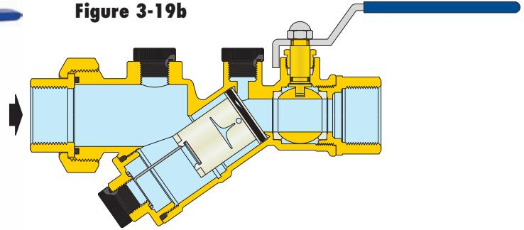
flow rates. Thus, flow rate through the valve will increase as differential pressure increases. The “inactive” position of the internal cartridge is shown in figure 3-20.
