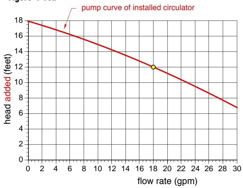
For our discussions, we will assume that the supply and return mains will be consistently sized for a nominal 4 feet of head loss per hundred feet of pipe. Using this assumption, the head loss across the mains at some location downstream of the circulator can be estimated as shown in figure 4-9.
