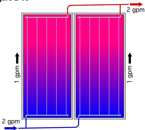
However, when more than two identical devices are piped in reverse return, the flow rates do not necessarily divide equally among all devices. To illustrate this, consider the reverse return piping assembly shown in figure 2-11.
