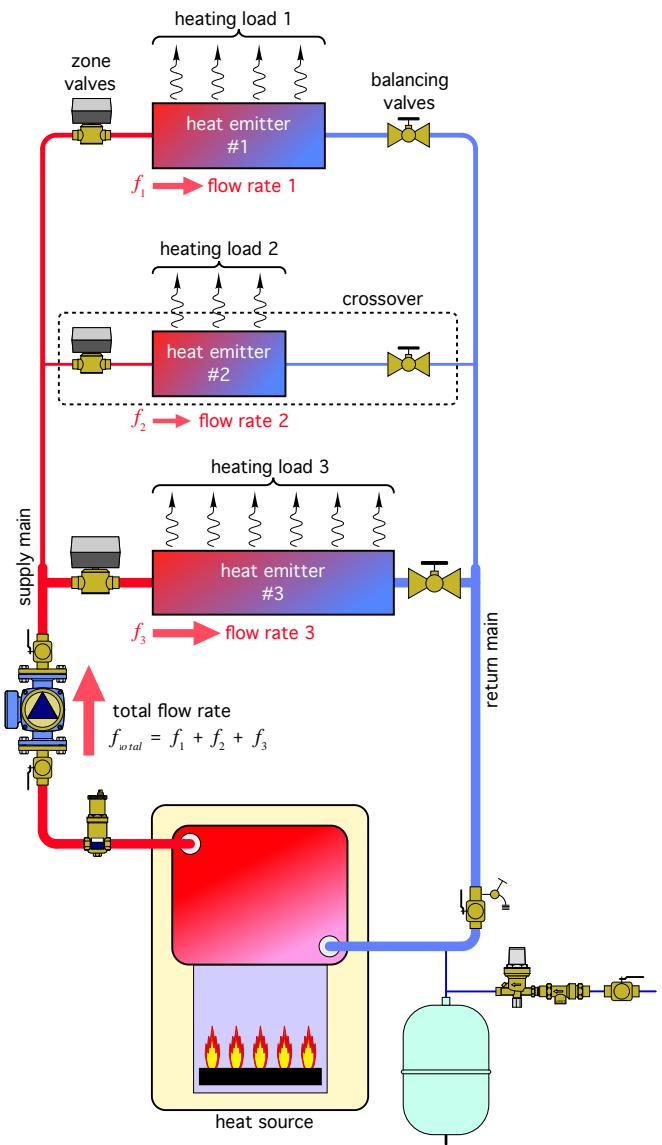
In some systems, two or more of the crossovers may contain the same heat emitter, or be piped with the same size and type of tubing. However, this is not always going to be the case. In the most general sense, every branch can contain different heat emitters, and different piping components.
