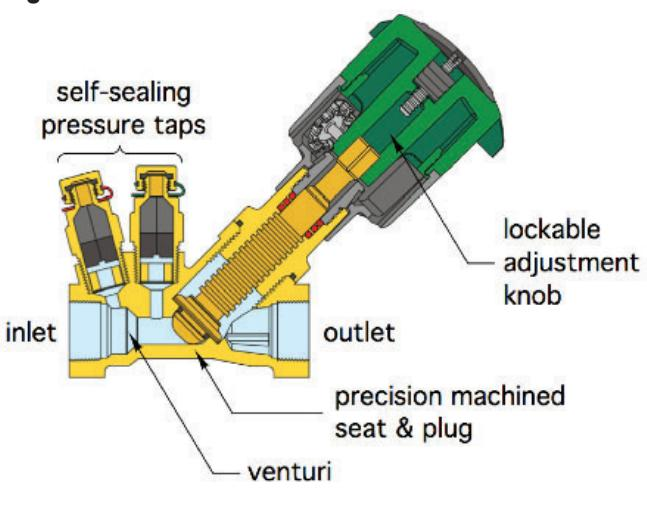
All valves with pressure taps require the use of a measuring instrument to read the differential pressure that infers the flow rate through them. An example of such a device is shown in figure 3-14.
