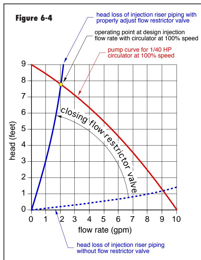
**Step 2:** Once the injection flow rate is calculated, turn on the injection pump at full speed. For AC circulators, this can be done by either setting the injection controller to full-speed mode or by wiring a line cord to the circulator and plugging it in. If a multi-speed injection pump is used, set it for the lowest speed setting.
