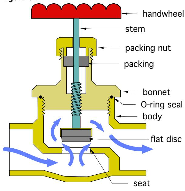
Globe valves should always be installed such that flow enters the lower body chamber, and moves upward toward the gap between the seat and disc. This allows the disc to close against the area of higher pressure. Reverse flow through this type of valve can cause unstable flow regulation, cavitation, and noise. All globe valves have an arrow on their body indicating the proper flow direction.
