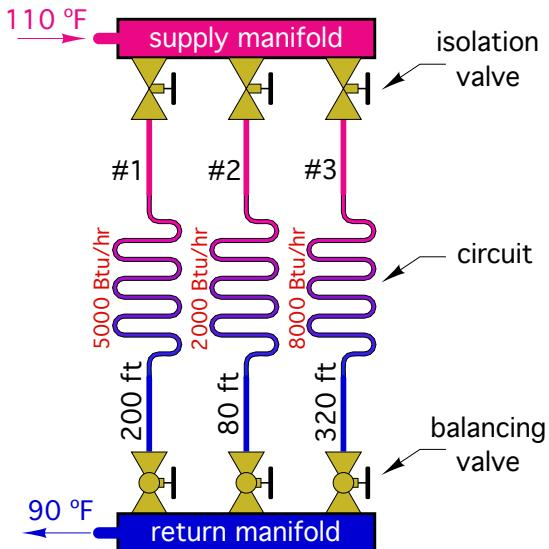
Assume three radiant panel circuits, each constructed of 1/2" PEX tubing, having the lengths and heat delivery requirements shown in figure 4-23.
