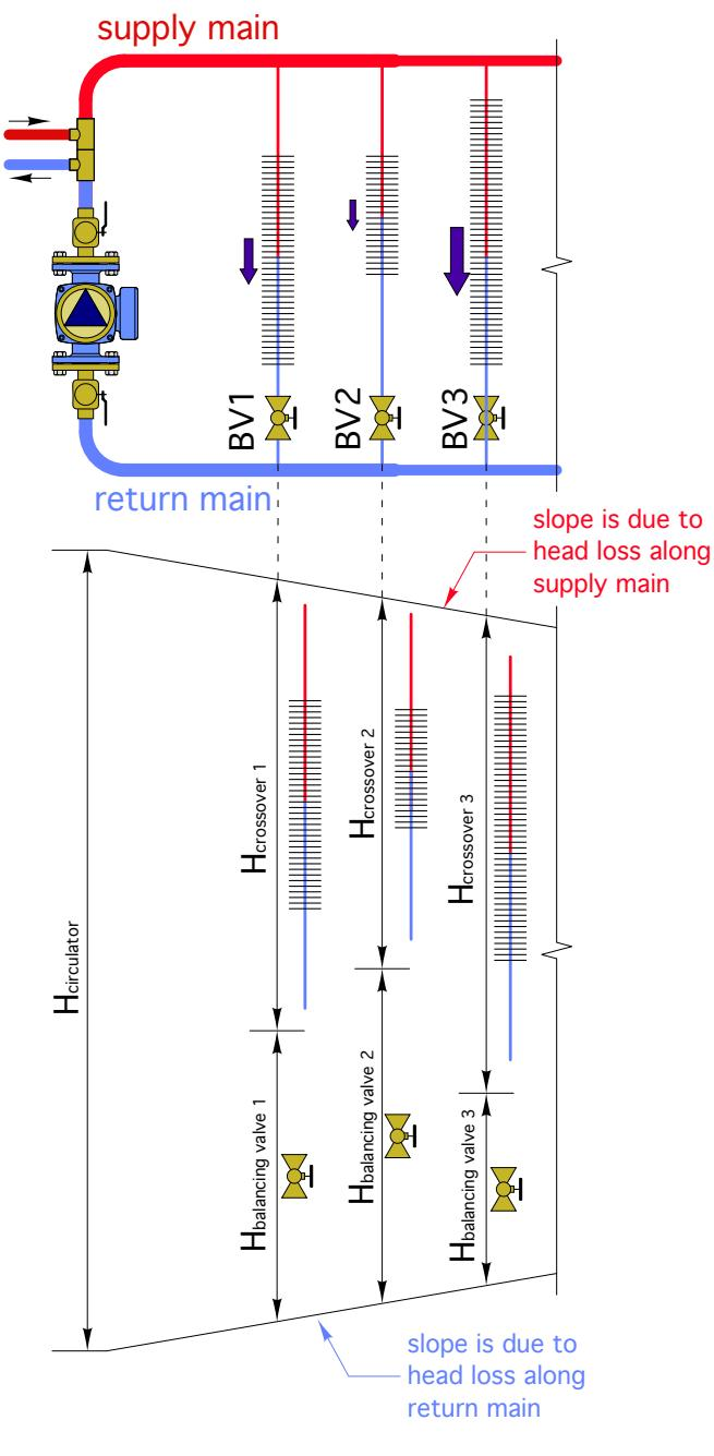
the mains. Less available head means lower differential pressure across the crossover, and thus lower flow rate. The head available to the “least favored crossover” at the far right of the system determines the flow rate through the crossover. In this system, the circulator is assumed to be sized so that it can provide the necessary head to drive flow through the least favored crossover, accounting for the head loss along the full length of the supply and return mains.
