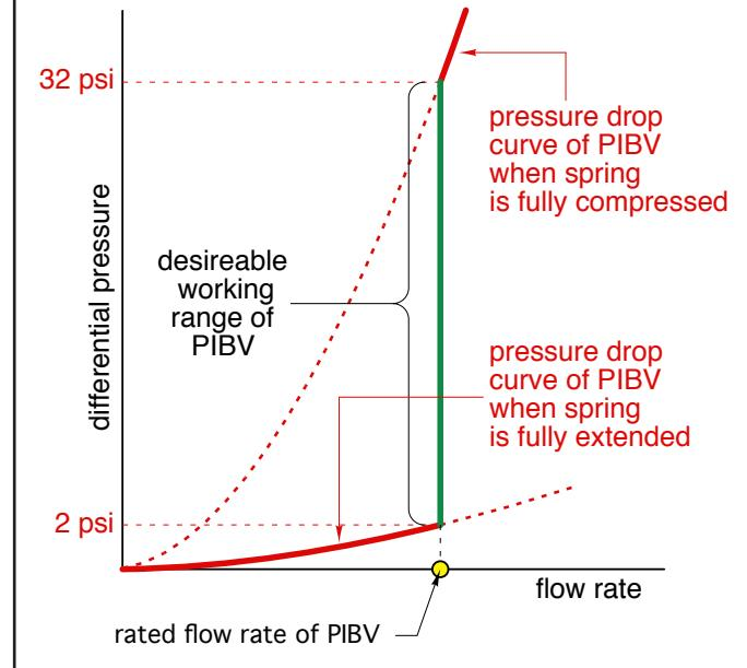
With a PIBV in each crossover, the flow rates through each *active* crossover remains at its design value, regardless of the flow status in other crossovers. However, this desirable condition is contingent upon keeping the differential pressure across the PIBV between its lower and upper threshold values. This condition is vitally important to proper application of such valves, and will be discussed further in section 5.
