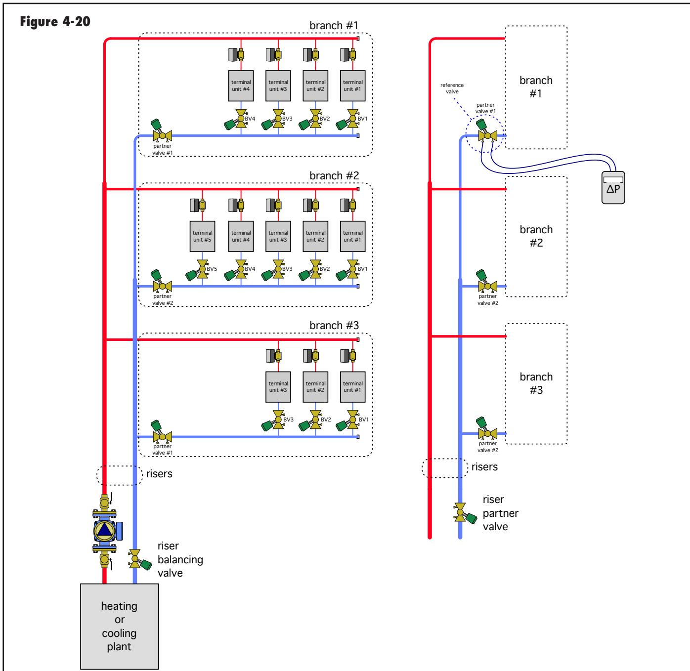
is then removed by adjusting the partner valve. When the balancing valves in all crossovers of the branch have been adjusted, all flow rates within those crossovers will change in proportion to each other, and the branch is considered “balanced.”
