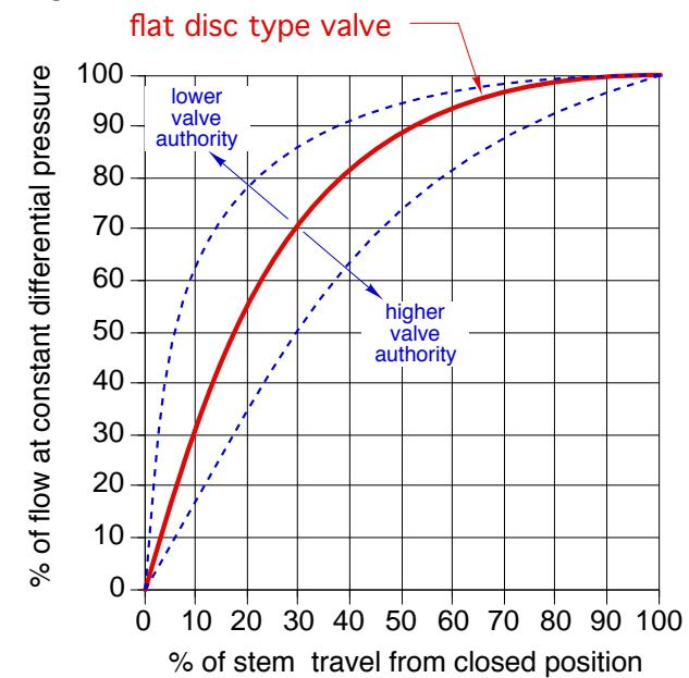
Notice that when the valve’s stem reaches the 50% open position, the valve is passing approximately 90% of the flow it will pass when fully open.
