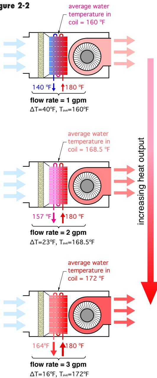
As the flow rate through the coil increases, the temperature difference between its inlet and outlet decreases. This means that the average water temperature in the coil increases, and so does its heat output. This holds true for all other hydronic heat emitters, such as radiant panel circuits, panel radiators and baseboard.
