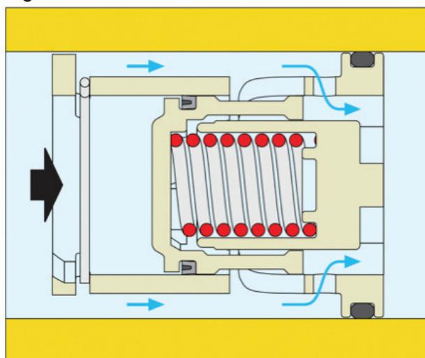
The unique polymer cartridges used in all Caleffi PIBVs are specifically designed for low flow noise.
