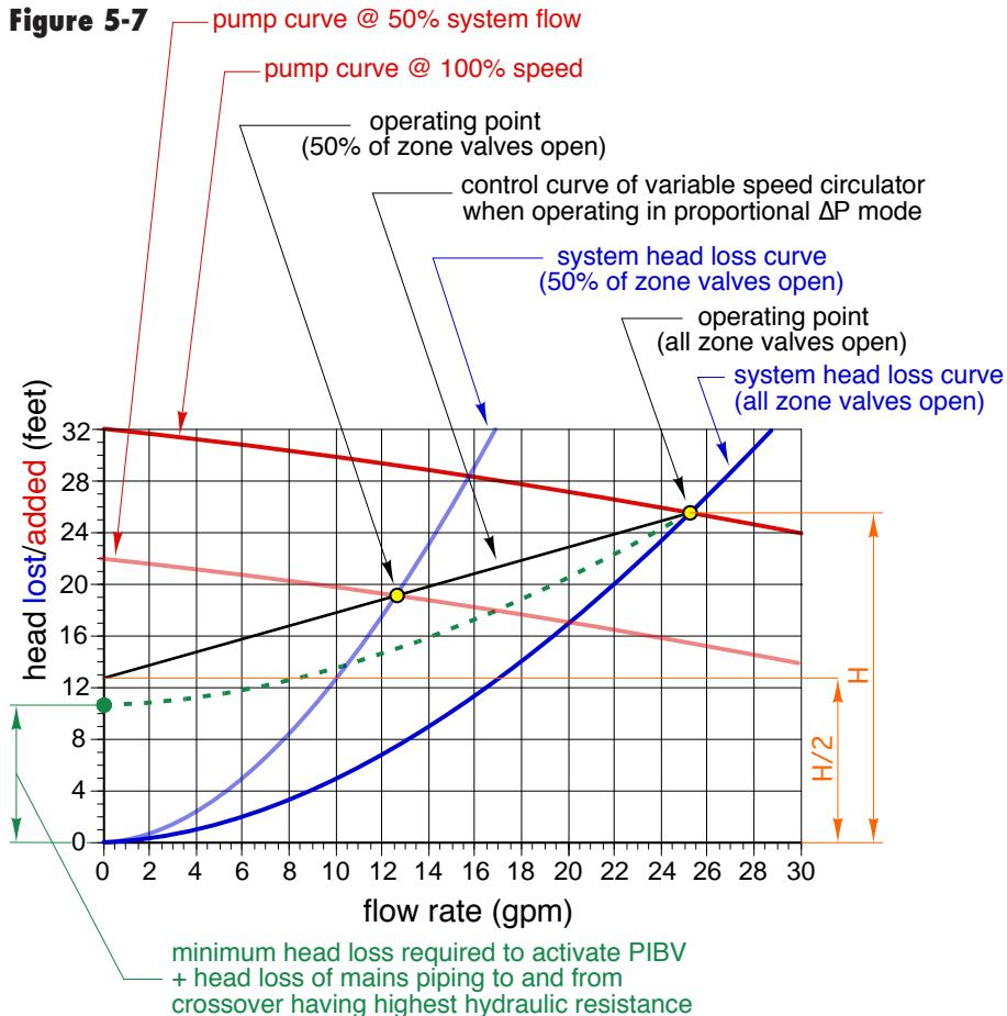
variable-speed circulator operates must not allow the differential pressure across the crossover with the highest hydraulic resistance to fall below the total of this minimum differential pressure plus the pressure drop of the other crossover piping components and piping mains when operating. The concept is shown in figure 5-7.
