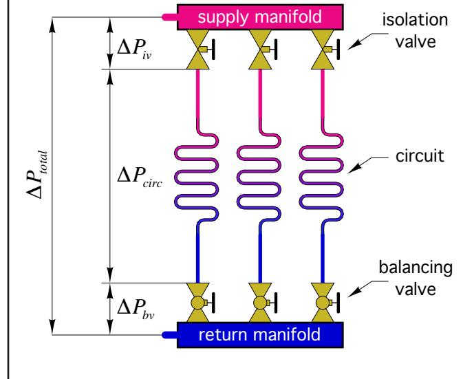
This diagram labels the pressure drop between the supply and return manifolds as  $\Delta P_{total}$ . This circuit with the highest pressure drop is found by combining the largest of the three circuit pressure drops ( $\Delta P_{circ}$ ) with the pressure drop through a fully open isolation valve ( $\Delta P_{iv}$ ), plus the pressure drop through a fully open balancing valve ( $\Delta P_{bv}$ ). This relationship is expressed as Formula 4-8.
