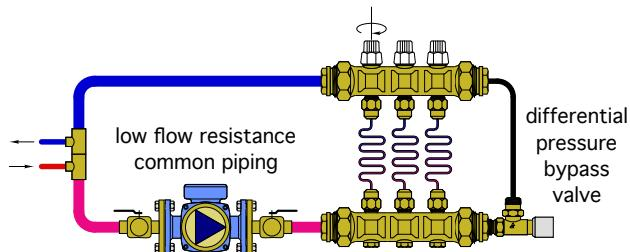
The converse is also true. Systems that lack differential pressure control, and/or have relatively high hydraulic resistance through the common piping, can create large changes in crossover flow rates when the flow through one crossover is adjusted. An example of such a situation is shown in figure 2-8.
