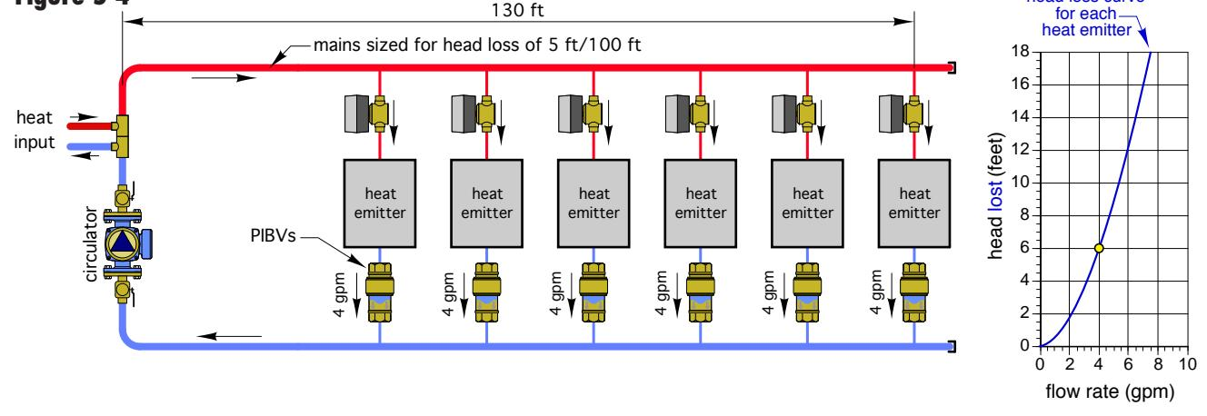
$$H_{L(\text{mains})} = \left( \frac{5 \text{ ft}}{100 \text{ ft}} \right) \times 2 \times 130 \text{ ft} = 13 \text{ ft}$$
