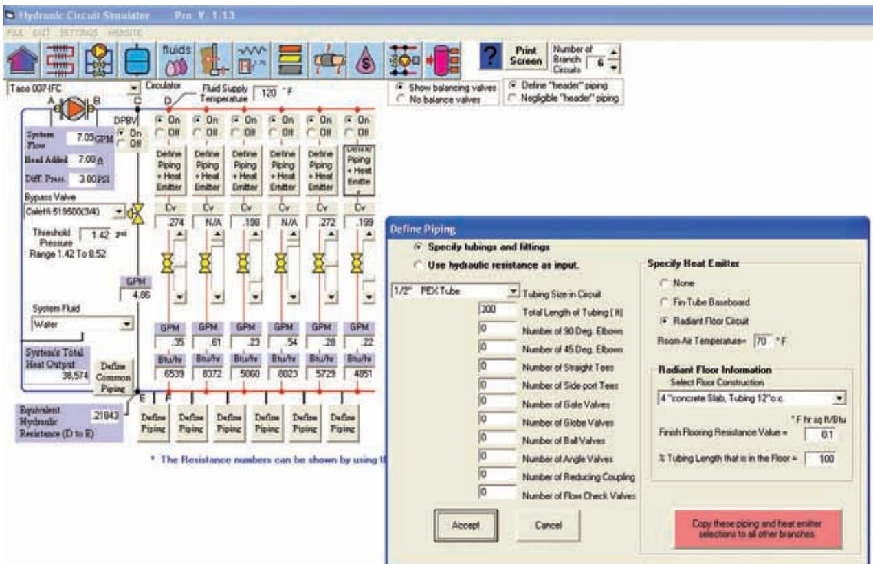
Figure 2-6 shows a screen from one software program that can simulate the thermal and hydraulic behavior of a multiple crossover hydronic system, including the effect of balancing valves and a differential pressure bypass valve.
