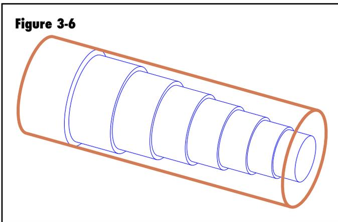
Because the water particles move in parallel streamlines during laminar flow, there is very little mixing between them. This increases the thickness of the boundary layer between the bulk of the fluid stream and the inner wall of the pipe. Thicker boundary layers decrease convective heat transfer.
