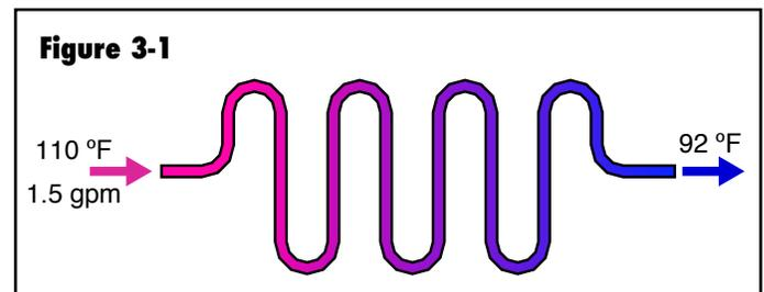
Solution: To use Formula 3-1, the density of water at its average temperature of 101°F must first be estimated using Figure 3-2:
