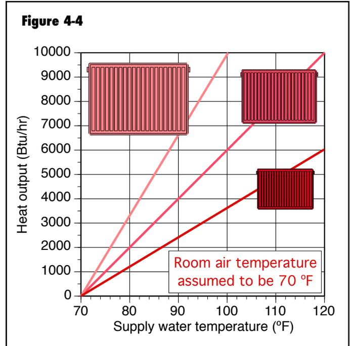
*The greater the total surface area of heat emitters in a system, the lower the required supply water temperature.*
