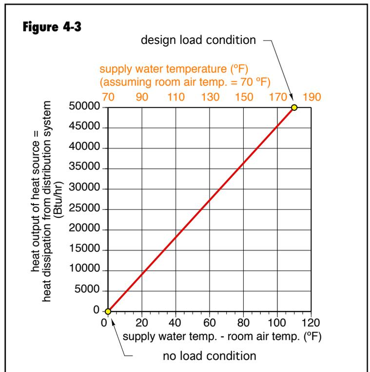
“pushes” heat from the water out through the heat emitters and into the room air.
