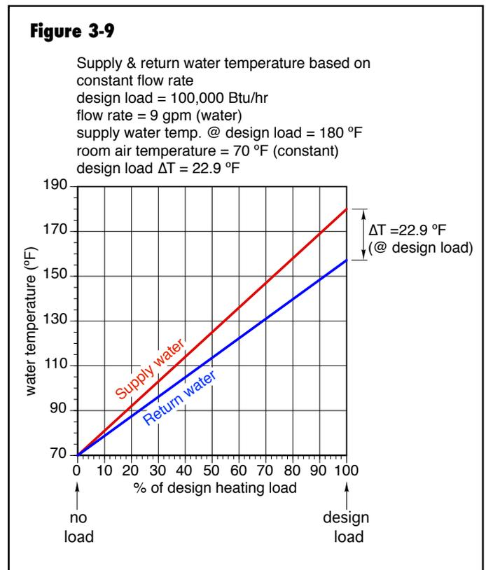
Although the value of the supply water minus return water ΔT will be different for different hydronic systems using different heat emitters, the relationship between supply
