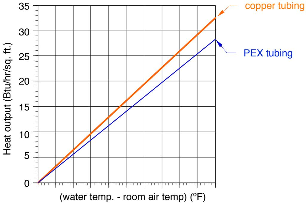
The thermal conductivity of the tubing options is:
