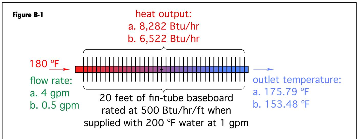
The total heat released from the baseboard can now be calculated using Formula B-2:
