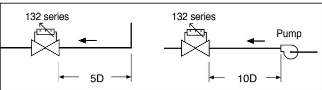
The valve can be installed in any position with respect to the flow direction shown on the valve body. Additionally, the valve can be installed either horizontally or vertically.
