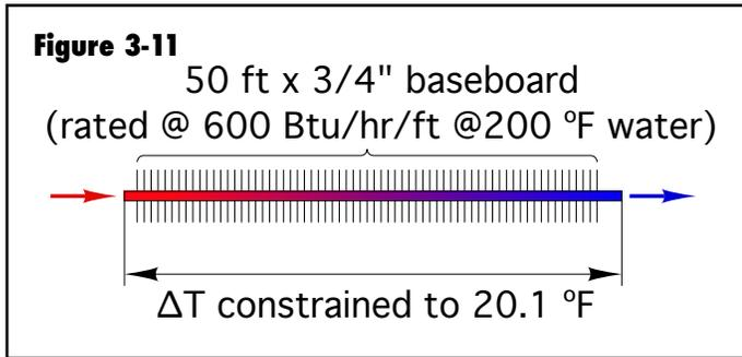
*This suggests that heat output under the combined effects of 1) reduced supply water temperature based on outdoor reset, and 2) constrained  $\Delta T$ , could result in inadequate comfort under partial load conditions.*
