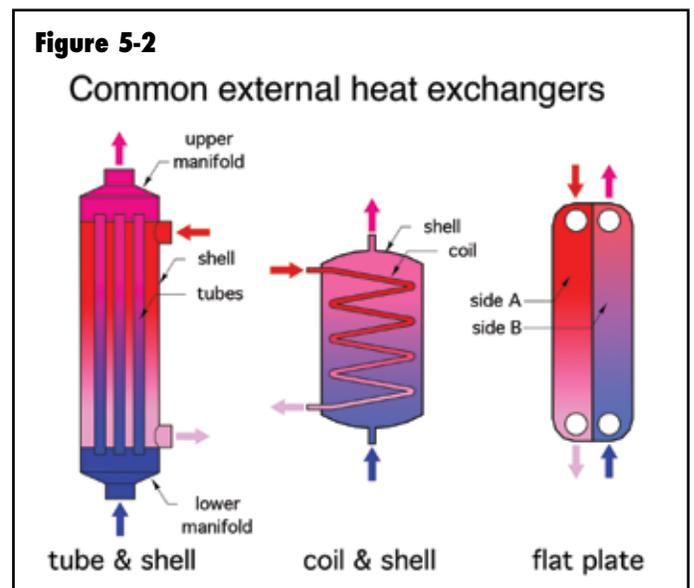
All external heat exchanger designs create two pressure-tight cavities that separate the fluids exchanging heat. They also create an internal surface across which heat moves by conduction through the metal separating the two fluids.
