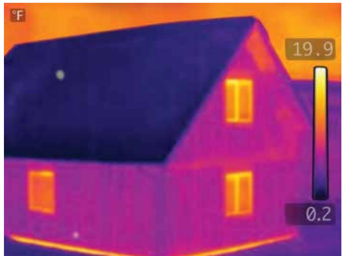
The rate thermal radiation transfers heat between two surfaces depends upon their temperatures, an optical property of each surface called emissivity, as well as the angle and distance between the surfaces.
