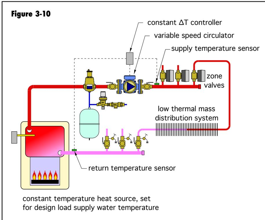
However, not all hydronic systems meet the three previously stated constraints. Many modern systems now use outdoor reset control to vary the water temperature supplied to the distribution system. When this method of water temperature control is combined with a controller that varies flow rate to maintain a *fixed*  $\Delta T$ , the heat output from the distribution system decreases faster than it should based on outdoor reset control theory.
