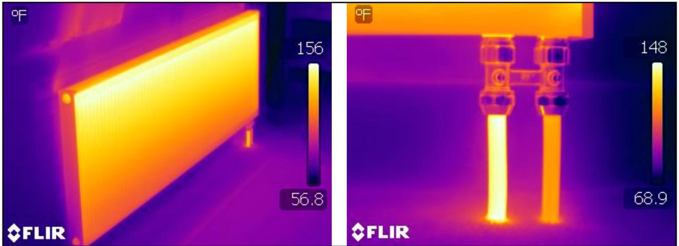
Notice the relatively even temperature gradient from the top to the bottom of the panel radiator. This indicates even flow distribution among the panels' vertical flow channels.
