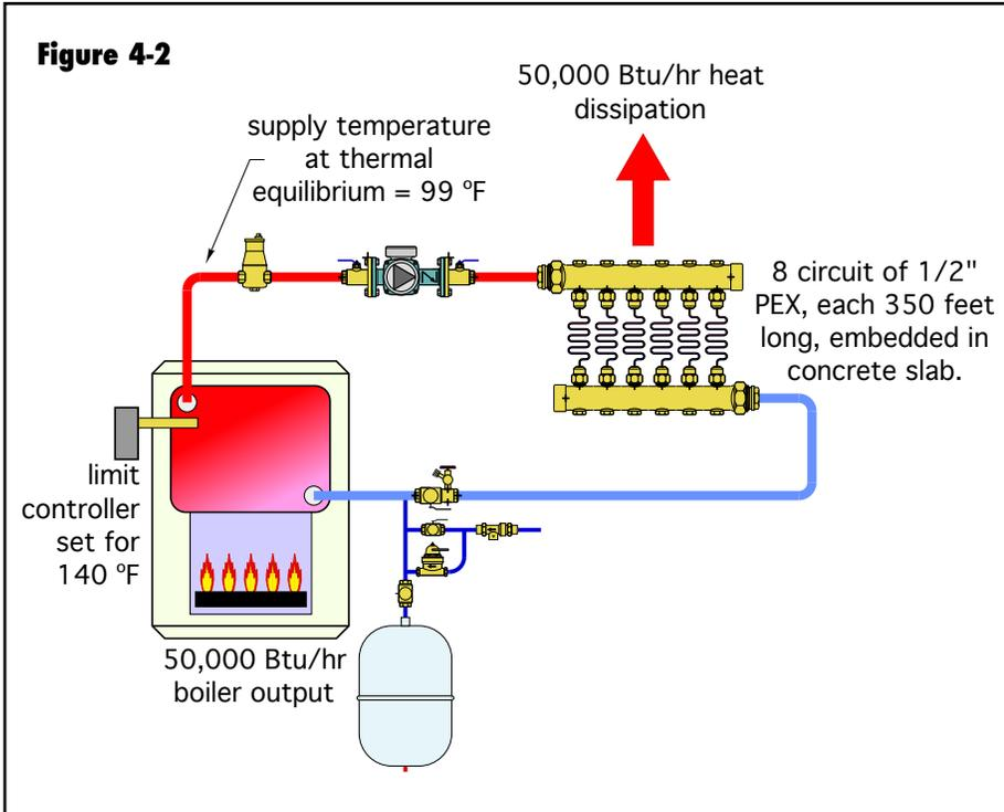
temperature at design load, and the total heat output of the distribution system at that same condition. This information should be determined as part of any accurate design process.
