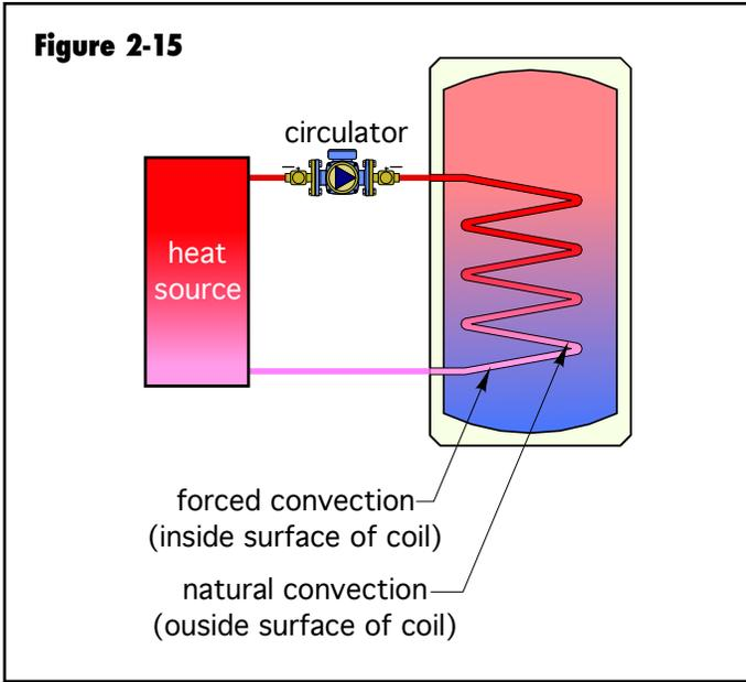
differences versus much faster motion created by a circulator. The slower fluid motion increases the thickness of the boundary layer, which creates greater resistance to heat transfer between the bulk of the fluid and the surface.
