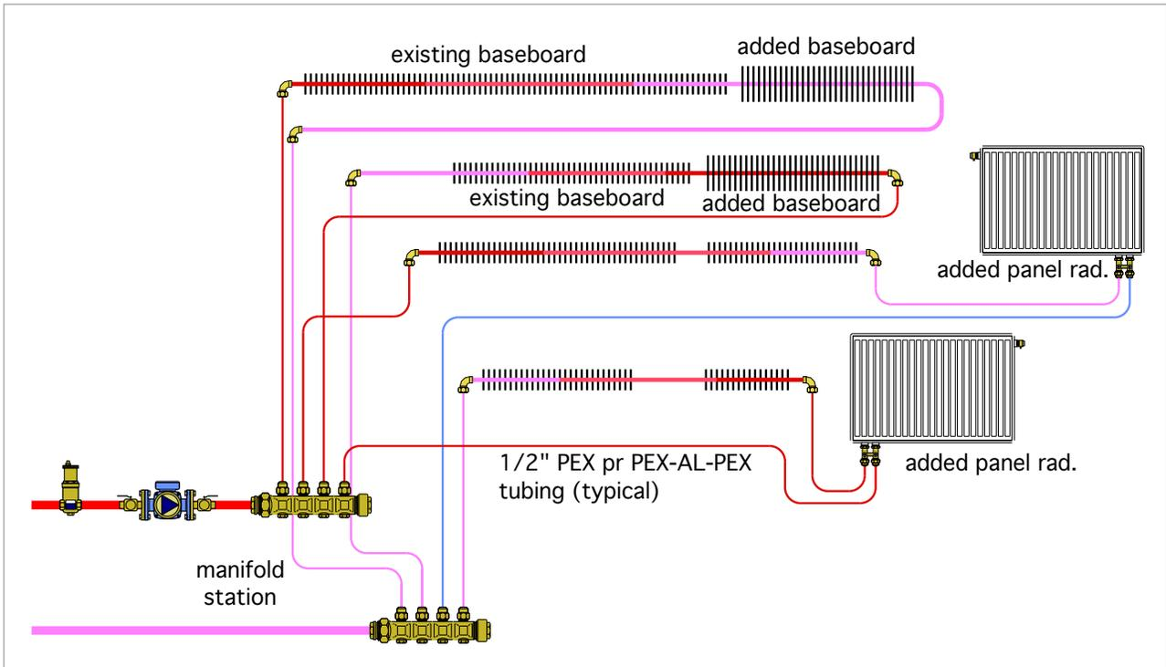
placement of the existing baseboard within each room. Designers should estimate the water temperature in the circuit at the location where the supplemental heat emitter will be placed, and size it accordingly.
