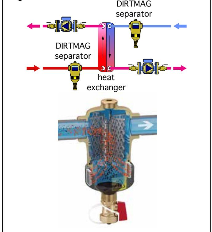
Caleffi DirtMag separators are recommended if either circuit passing through the heat exchanger contains components made of carbon steel or cast iron, both of which can be a source of magnetite. DirtMag separators are also recommended if a circulator with a permanent magnet motor (e.g., ECM) is used in either circuit. Figure 5-15 shows a Caleffi Dirtmag separator with the magnet removed, and being “blown down” to eliminate iron oxide (magnetite) from the system.
