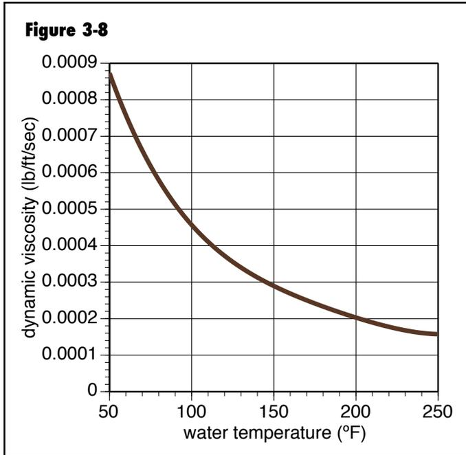
At 140°F, the density of water is 61.35 lb/ft<sup>3</sup>. From Figure 3-8, the dynamic viscosity of water 140°F is 0.00032 lb/ft/sec.
