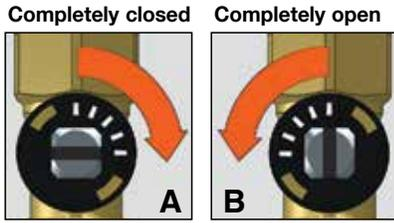
For the flanged version, rotate the adjusting handwheel 90° for the complete opening and closing of the valve as shown in (A) and (B). When at the desired position, lock the adjustment screw.
