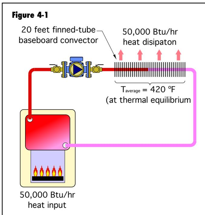
Assume that there are no controllers in this system, no pressure relief valve, and that all components used have very high temperature and pressure ratings. Also, assume that the room air temperature is 70°F.
